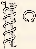
FIG. 1. Probable method of making links for mail.
